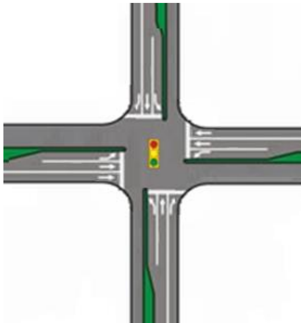
Figure 15: Signalized Intersection (2-Lane Major Street Approach)
