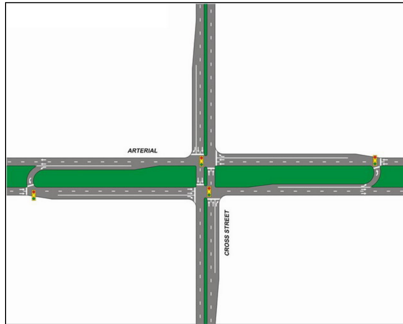
Figure 1 Typical median U-turn intersection (UMD, 2004)
