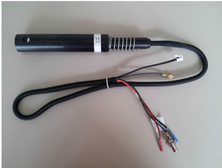
Figure 3.20 A pixel from the upgraded VERITAS II cameras.
