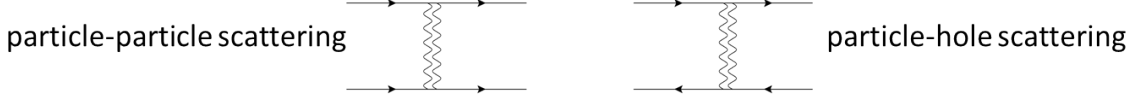
Figure 3.3 Diagrammatic demonstration of the effective particle-particle and particle-hole interaction by the exchange of fluctuations. The double curved line refers to the renormalized fluctuation propagator and the single line represents single-particle propagator.
