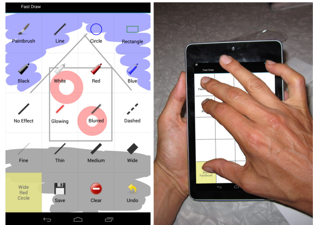
Figure 6. Left: transparent grid with drawing behind. Right: three-finger chord that selects two commands.
