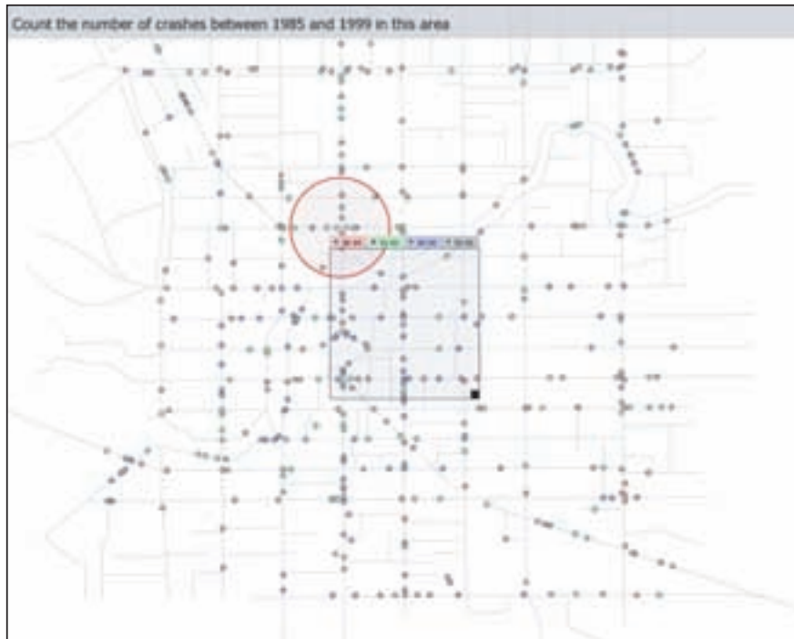
(c) The Magic Lens interface combines the Static View with filtering. Filtering only occurs within the lens area and is controlled with checkboxes attached to the lens.
