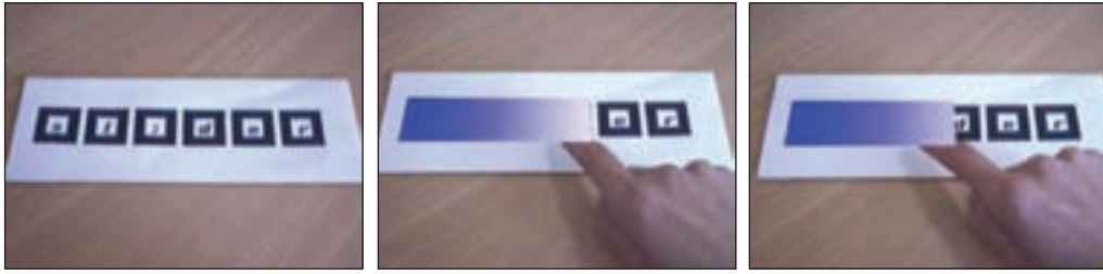
Figure 7.3: Occlusion selection technique for marker-based AR by Lee et al. (2004). In this example, a rudimentary slider is implemented by determining which markers in the row are currently blocked from the camera. Image courtesy of Gun Lee.
