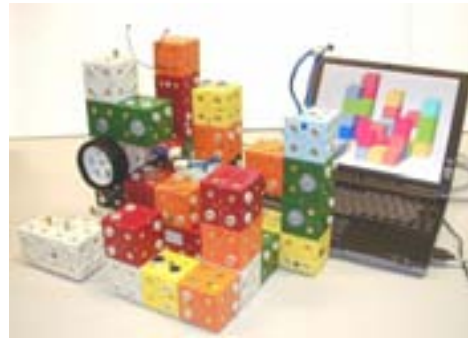
(b) ActiveCubes can be connected together into 3D structures interpreted by the computer.
