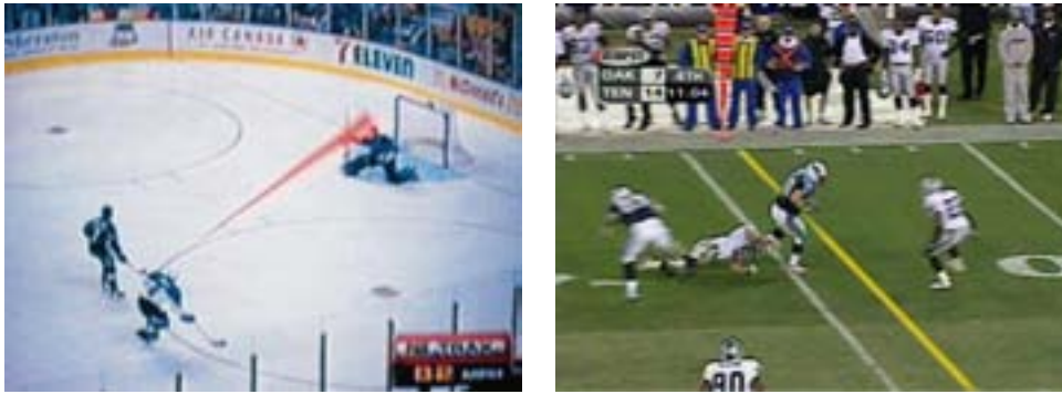
(a) Ice hockey puck with virtual comet trail. (b) The virtual first down line in American football.
