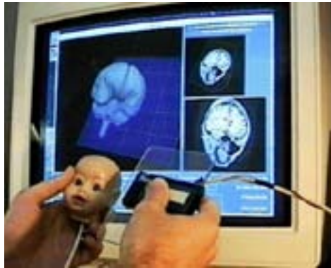
(a) Selecting a cutting plane with tangible props. Image courtesy of Ken Hinckley.
