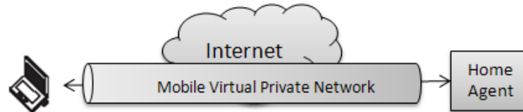
Figure 9-7 Mobility without infrastructure support - Road Warrior
