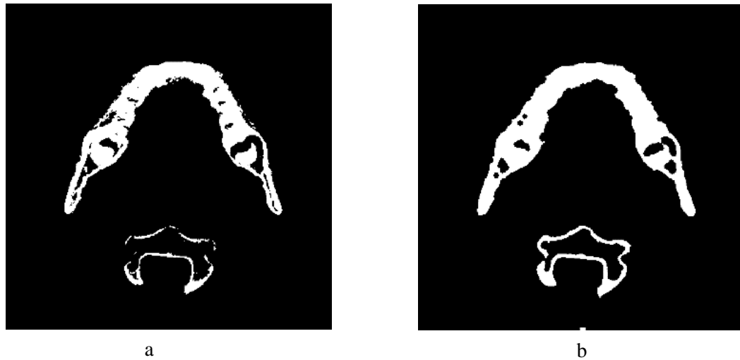
Figure 4.8. Illustration of denoising process. (a) Binary image (noise present), (b) Denoised image after morphological filtering.
