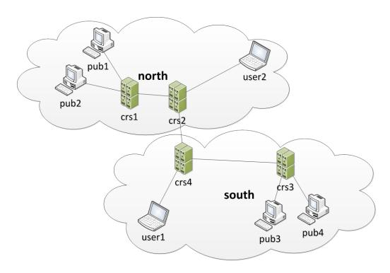
Figure 7 Emulab Inter-domain experiments topology
