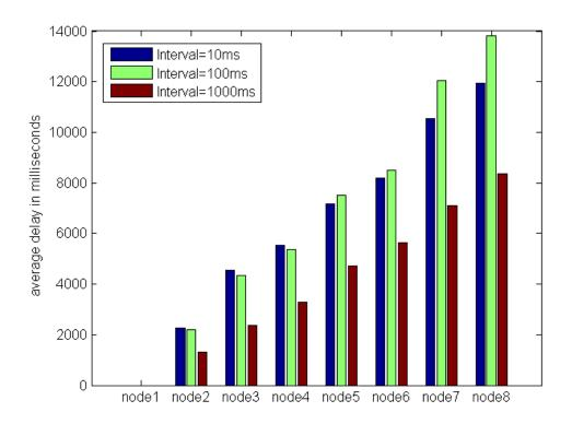
Figure 11 hop by hop delay for 256KB data content
