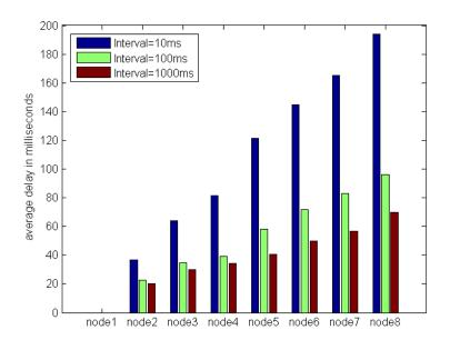
Figure 9 hop by hop delay for 1KB data content
