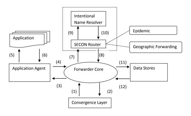
Figure 2 intentional name resolution data flow
