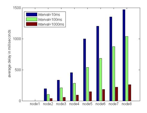
Figure 10 hop by hop delay for 16KB data content
