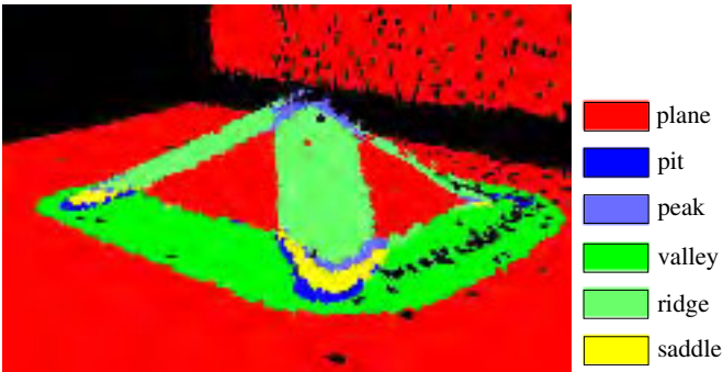
(b) Discontinuity/crease removal and surface type classification.
