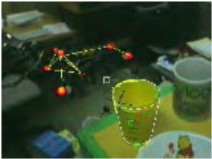
(b) Hybrid visual servoing after gripper enters view
