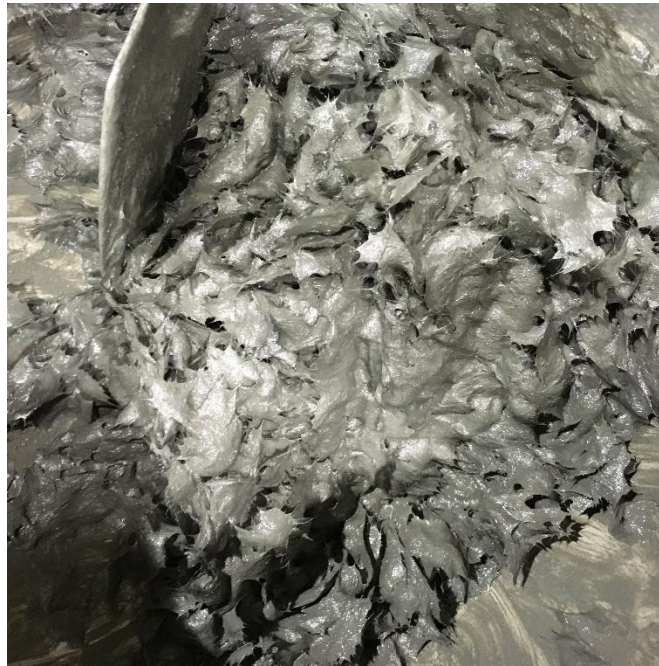
Figure 5-14 Bad workabilities during the fabrication of samples with 1.5% CF content
