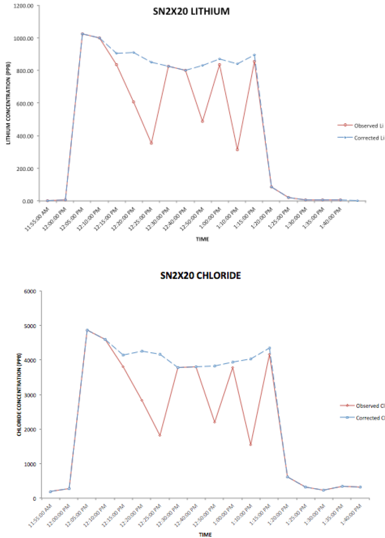
Figure 3-17. Observed lithium BTCs shown with corrected BTCs and sulfate comparison at SN2X20
