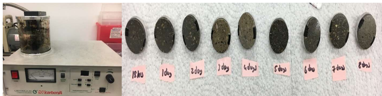
(a) (b) Fig 3.1: a) carbon sputter, b) samples mounted on sample stub
