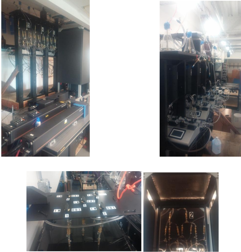
Figure 19: Physical setup of EIE experiment. Optics bench, EIE frame, and fluid conveyance system front panel (top left). Fluid conveyance system back panel and syringe pumps (top right). EIE cell coupling to fluid conveyance system (bottom left). EIE apparatus imaging window as seen from underneath (bottom right).
