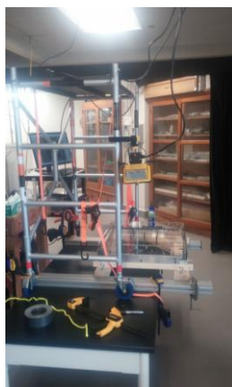
Figure A5: EIE suspension equipment for HCP bead loading.
