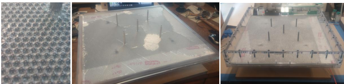
Figure A4: 3mm beads in HCP configuration topped with 1mm beads (left), bead loading rig in extended position and packed with beads (middle), EIE cell aligned with bead loading rig prior to bead placement within the EIE apparatus (right).
