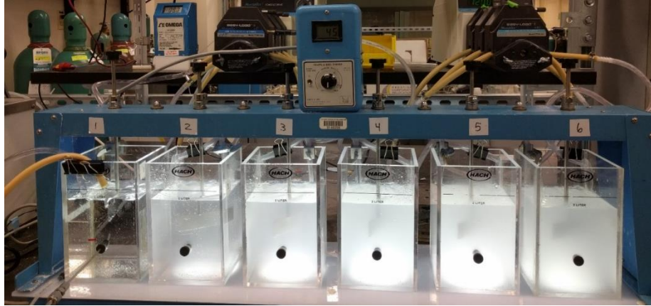
Figure 9- Six CSTRs running in steady state (individual residence time, \tau = 11.3 min).
