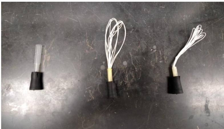
Figure 4- HFM aeration device and plain bubbling tube. [14]
