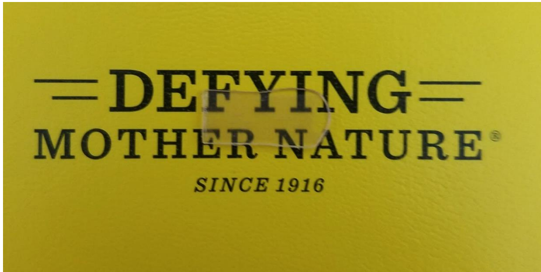
Figure 4. Transparent wood composite sample created by Kyle Foster.
