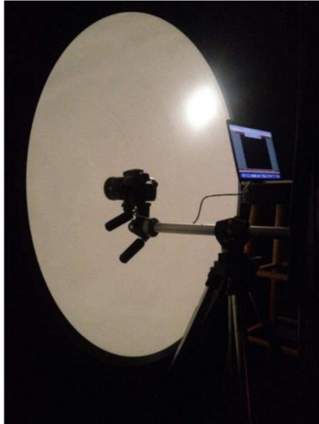
Figure 40: Integrating sphere set-up with camera in place
