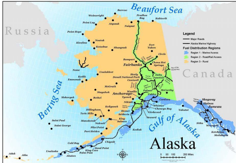
Figure 2: The road system and fuel distribution areas of the state of Alaska. Only region 2 (in green) has road and rail access. Region 1 (blue) is served primarily by the Alaska Marine Highway and air services. Region 3 (yellow) is exclusively accessible by coastal or river boat or barge, air services, and off-road trail or snow vehicles (Alaska Department of Environmental Conservation 2017a).
