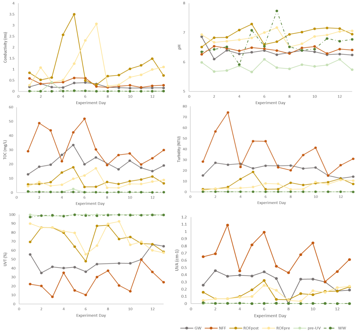
Figure 11: Conductivity, pH, TOC, turbidity, UVT and UVA in samples from six different points in the wash water treatment system during the whole household viral challenge with MS2.
