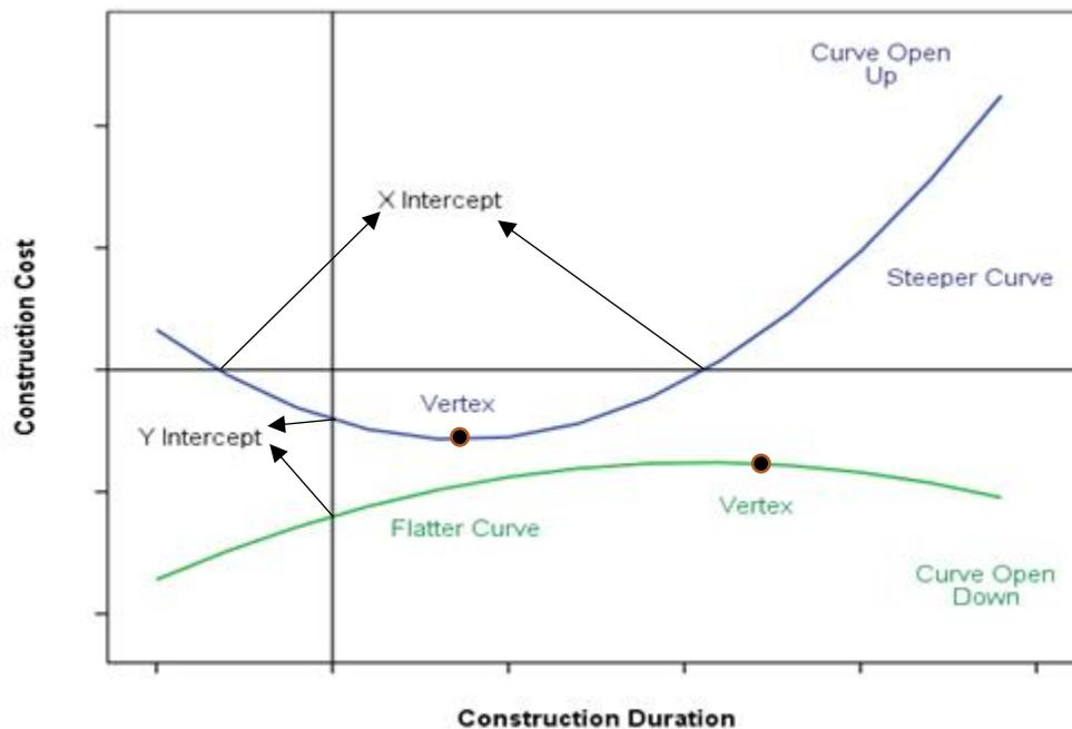
Figure 3: Properties of the second-degree polynomial curve
