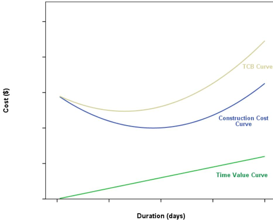
The TCB equation represents the total cost of construction process from the public's point of view. Contractors should generally minimize the TCB value in their offers to increase their chances to win new projects. The TCB equation is obtained by adding the construction cost equation to the time value equation and is given in equation 15 below:
