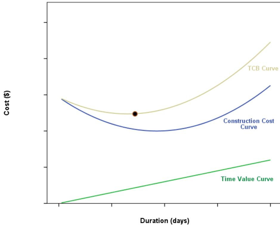
Ideally, the optimum price-time combination is the point where the TCB value is minimized. This point can be determined by taking the derivative of equation 15 or by looking directly on the TCB curve. Contractors could also use the TCB curve to look at different price-time combinations and then pick the most suitable one for them.
