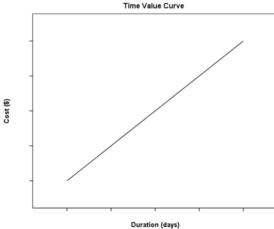
The time value (TV) curve represents the indirect costs or the loss of money that may be caused by the construction process. Usually the time value equation is determined by multiplying the unit time value (UTV) by the construction duration as given in equation 14. The UTV is normally given in the contract appendix and is usually equals to the daily road user cost (DRUC) in highway projects.
