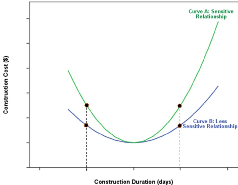
Figure 4: Construction cost and duration relationship sensitivity
