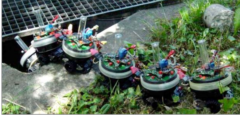
Figure 1.28: Chain formation for a narrow passage [112]
