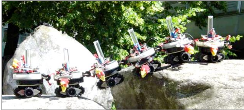
Figure 1.27: Holes avoidance through group reconfiguration [112]
