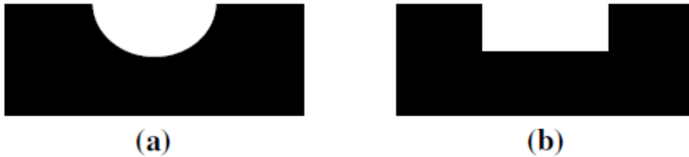
Figure 4.8: A schematic of an (a) isotropic etch profile and (b) anisotropic etch profile.
