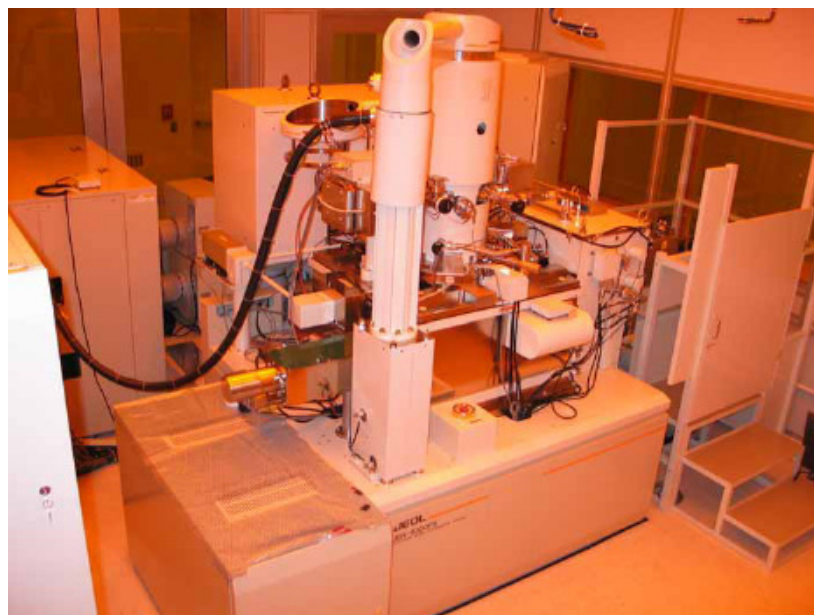
Figure 3.4: JOEL JBX-9300FS Electron Beam Lithography Tool for patterning electron-sensitive resist.
