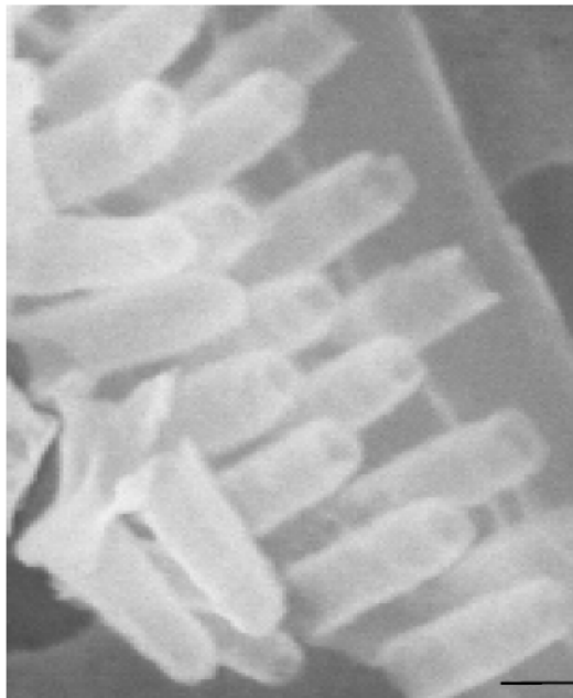
Figure 8.3: FE-SEM of 100 nm diameter PZT tubes, with ~15 nm wall thickness, mechanically removed from the underlying substrate and appended to a microprobe tip (scale bar 100 nm).
