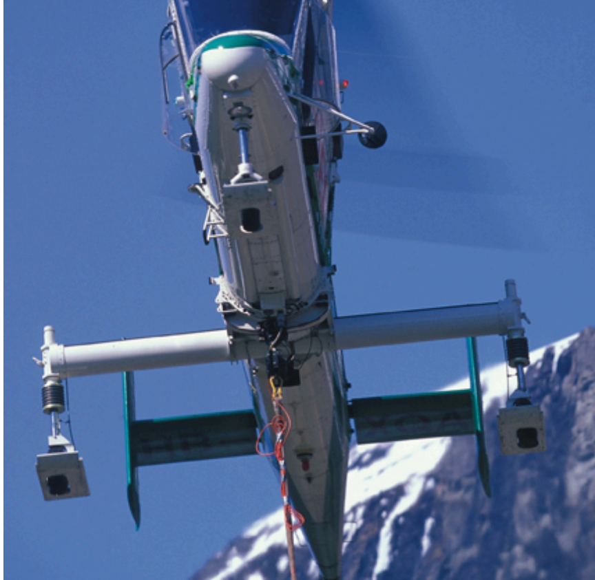
Figure 8: Underside of the K-MAX ® helicopter showing the suspension point sliding-rail mechanism 7 .
