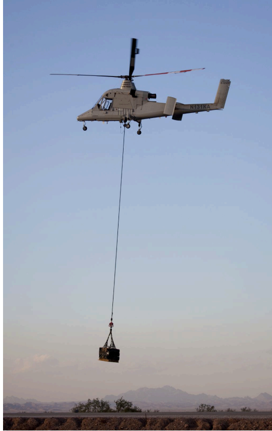
Figure 4: Unmanned K-MAX ® helicopter transporting cargo during a demonstration to the U.S. Marine Corps 5 .
