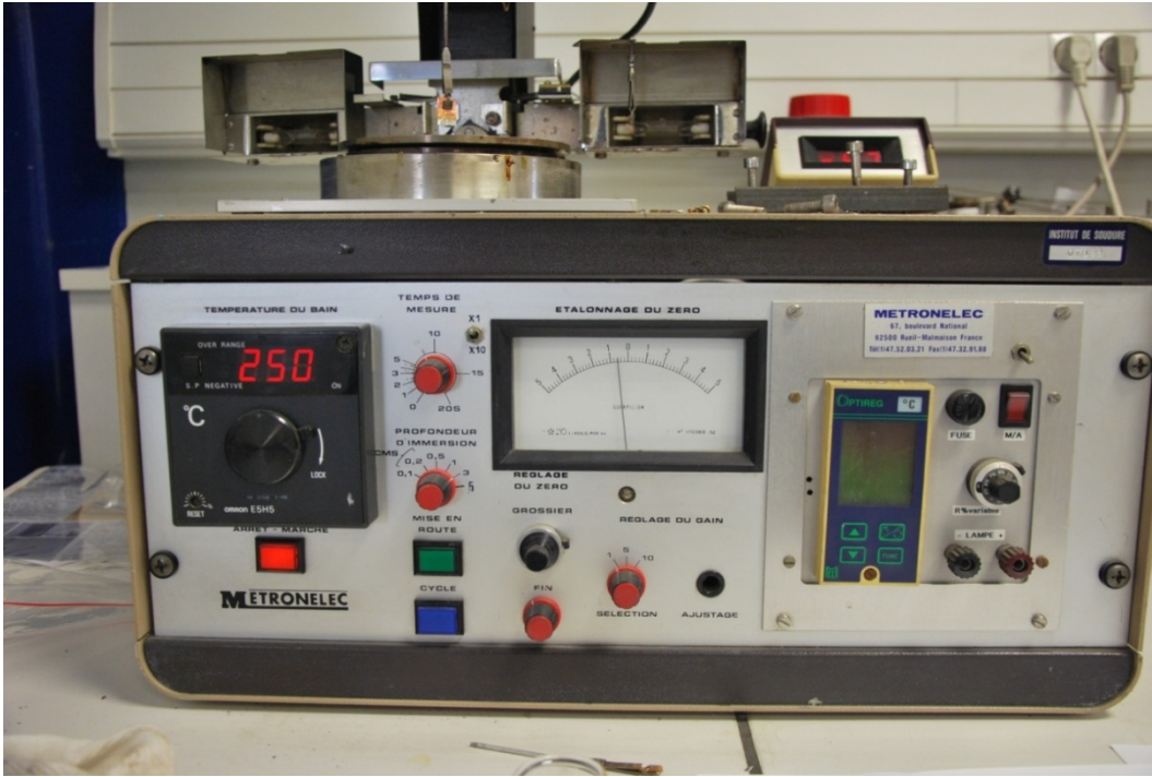
Figure 9.7: METRONELEC wettability setup
