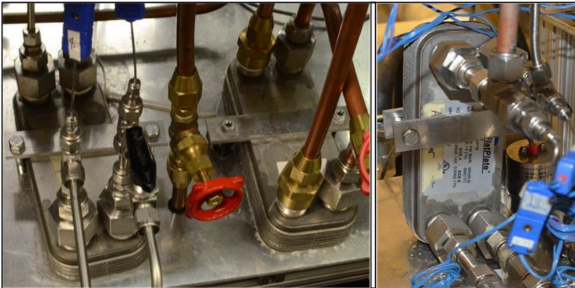
Figure 4.5: Solution Heat Exchanger and Absorber CF Heat Exchanger (Left) and Absorber (Right)
