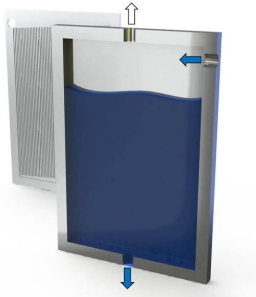
Figure 1.10: Flooded Column Desorber (Image Courtesy of Jared Delahanty)
