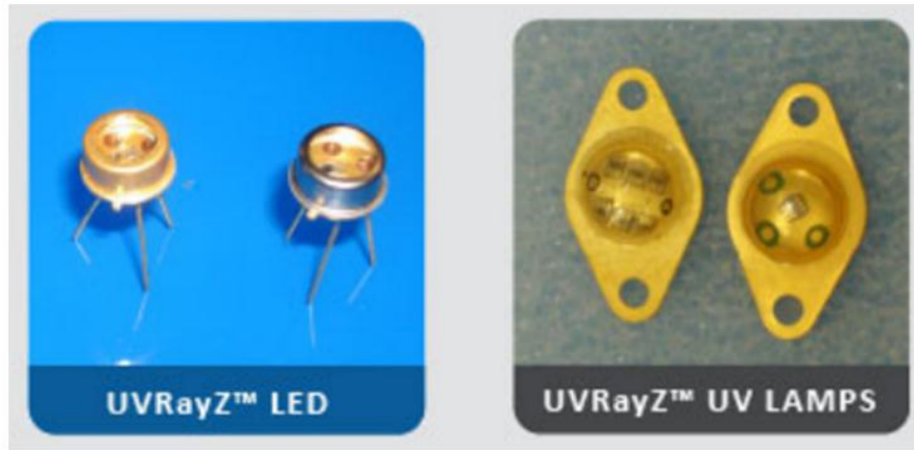
Figure 2.3 TO39 packaged UV LEDs and TO3 packaged UV Lamps offered by Nitek Inc [38].
