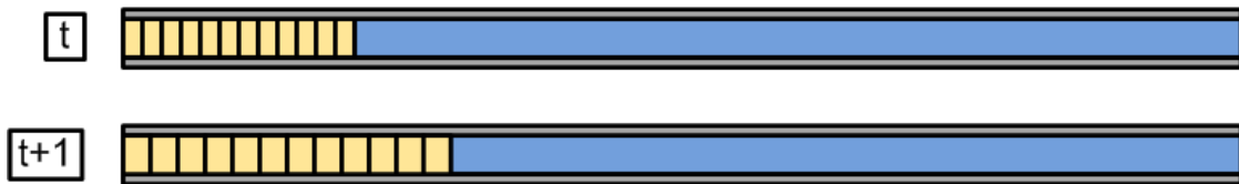
Figure 3.11: Illustration of the axial discretization scheme for two consecutive time steps. The control volumes in the gas region change size such that a discrete, well-defined boundary always exists at the liquid-gas interface.
