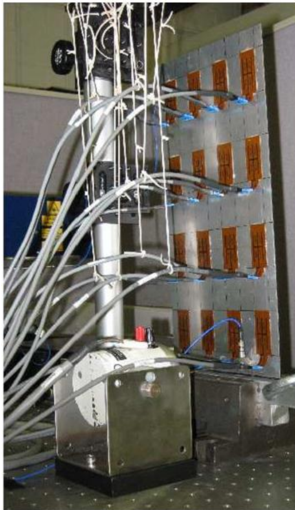
Figure 6.15 - Finite periodic assembly used to experimentally validate the effectiveness of hybrid shunting
