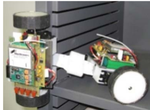
Figure 5.6 Twist / bend for direction change on different surfaces.
