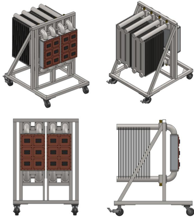
Figure 4.5. 5kW to 40 °C Design a) Front isometric b) Rear isometric c) Front view d) Side view
