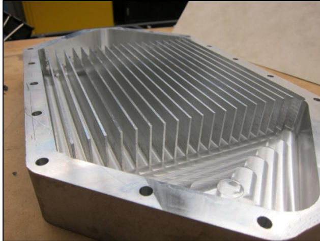
Figure 3.9 Machined hot side flow channels
