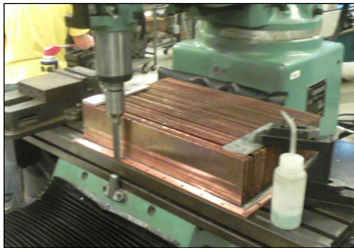
Figure 5.4 Machining of hot side fin array mounting flange
