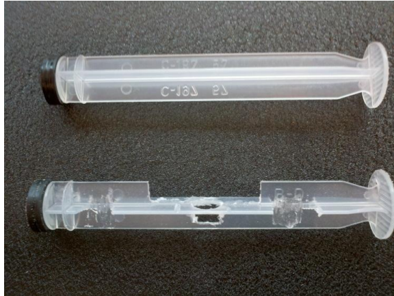
Figure 29. Plunger before and after modifications
