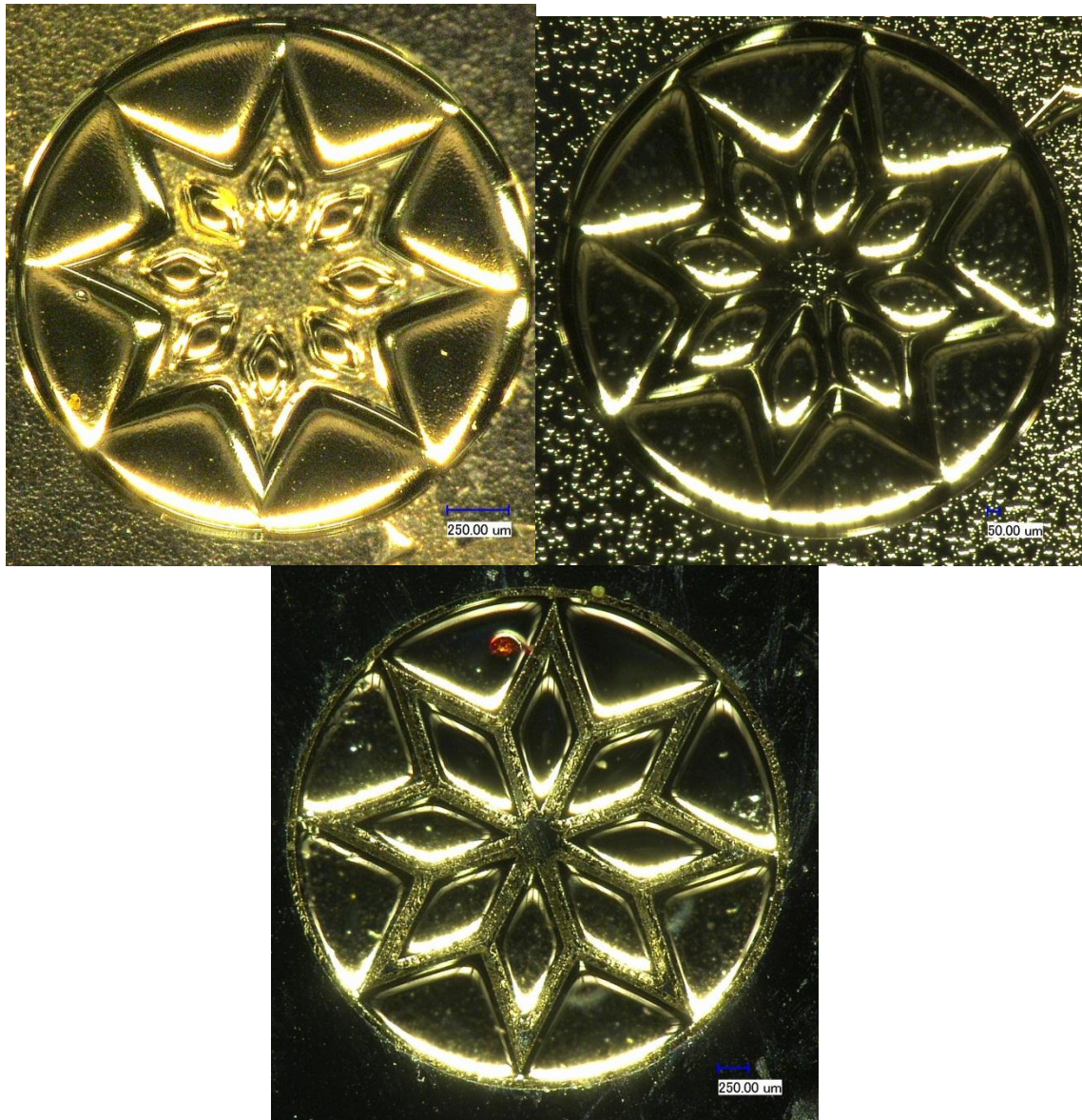
Figure 5.6 Optical micrographs of 2 mm CTC cavities in Si: 50%, 60%, 70% PCM fraction (clockwise from top left)
