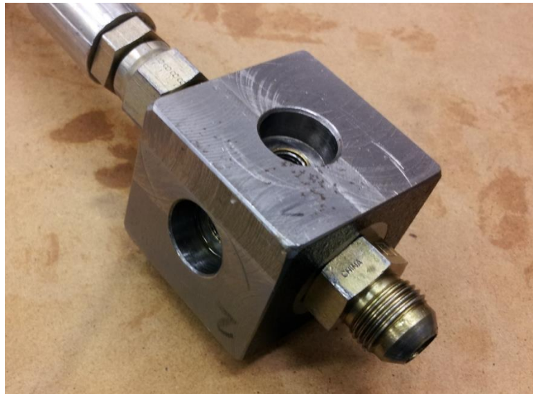
Figure 7: Calibration block without sensors
