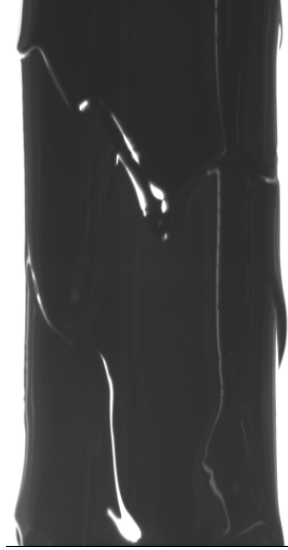
Figure 6.14: Experimental black liquor ( \chi_s = 0.41 , T = 298.15 K) falling film free surface waves.
