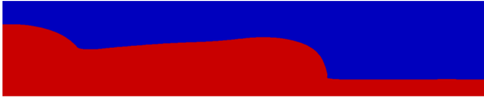
Figure 6.16: Black liquor film free surface waves ( \chi_{s,in} = 0.50 , Re = 50 ) showing large amplitude waves traveling downstream over a preceding flat thin liquid film.
