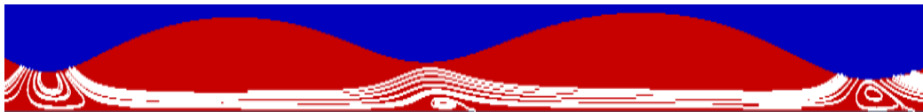
Figure 4.17: Normalized liquid film streamwise pressure gradient ( p_x = \frac{\partial p}{\partial x} )/ \gamma and normalized interface height \delta/\delta_N for flow conditions corresponding to solitary-capillary-capillary waves interaction.
