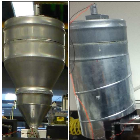
Figure 5.4 - Hopper Assembly Free From and Supported by Modified Duct
