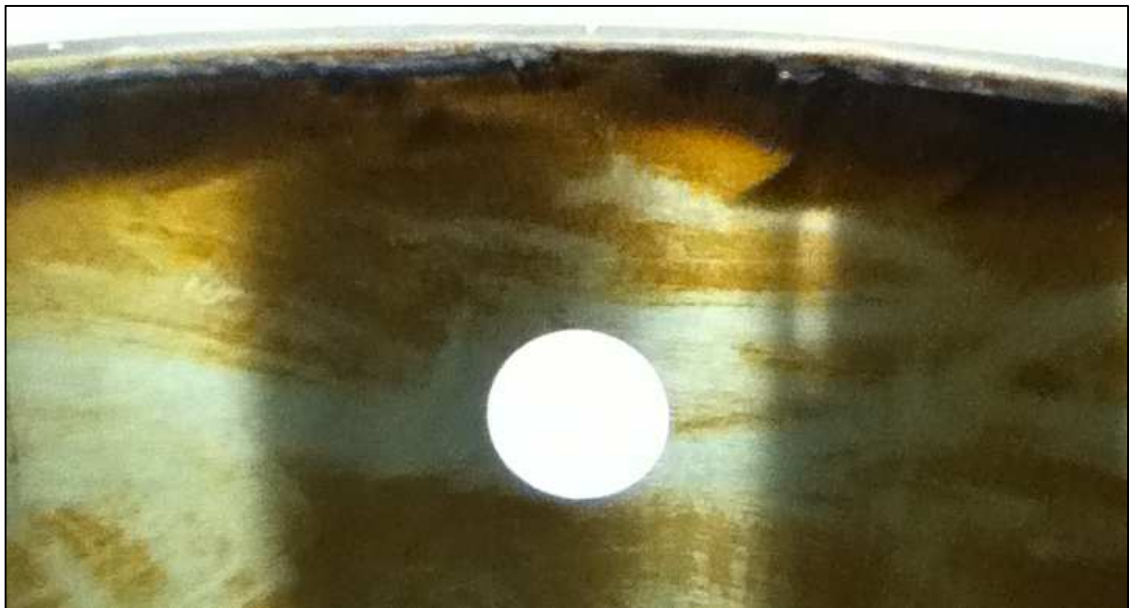
Figure 5.25 - Tar Formation on Reactor Chamber Walls
