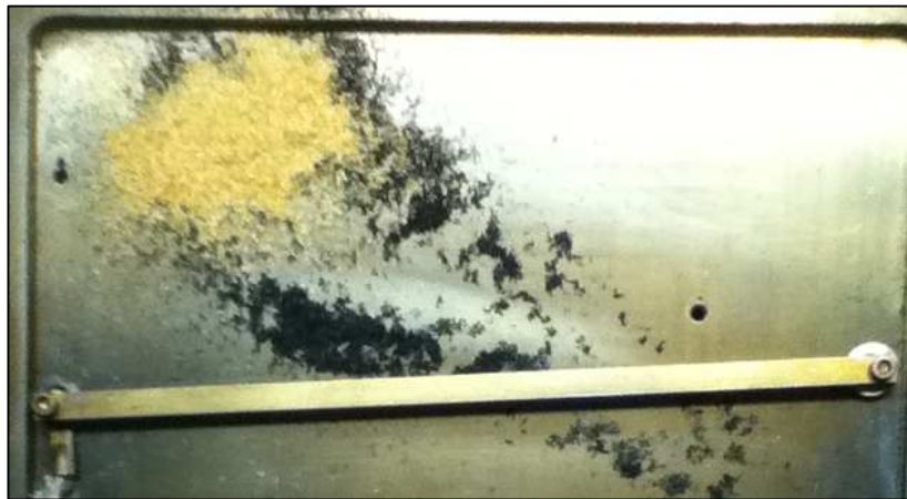
Figure 5.28 - Unreacted Biomass Buildup on Residual Char Layer in Experiment with Top Spreader Removed
