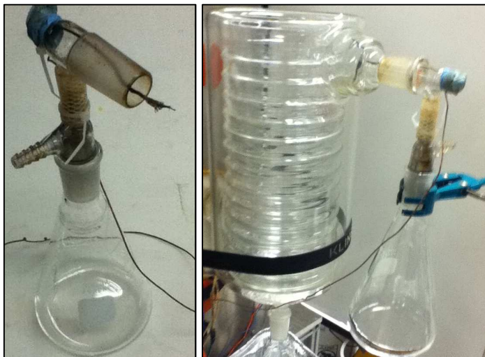
Figure 5.9 - Secondary Flask Assembly Free Standing and Attached to the Condenser Assembly
