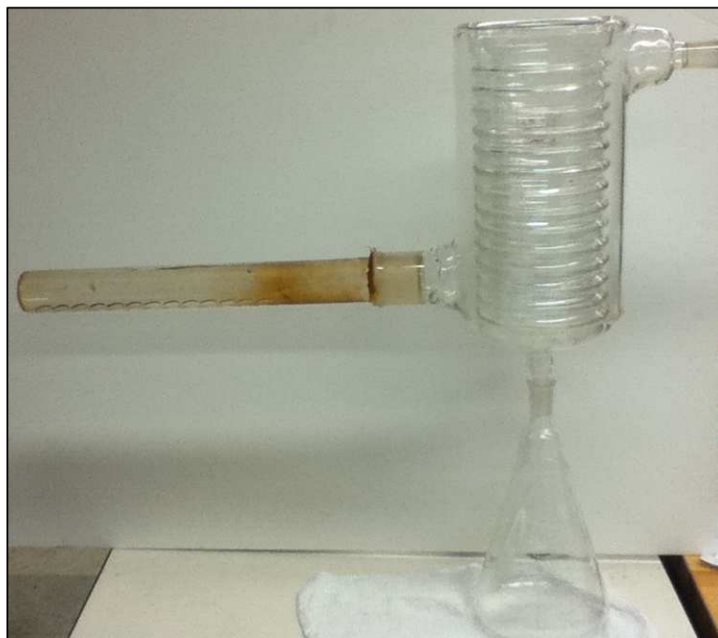
Figure 5.7 - Primary Condenser Assembly
