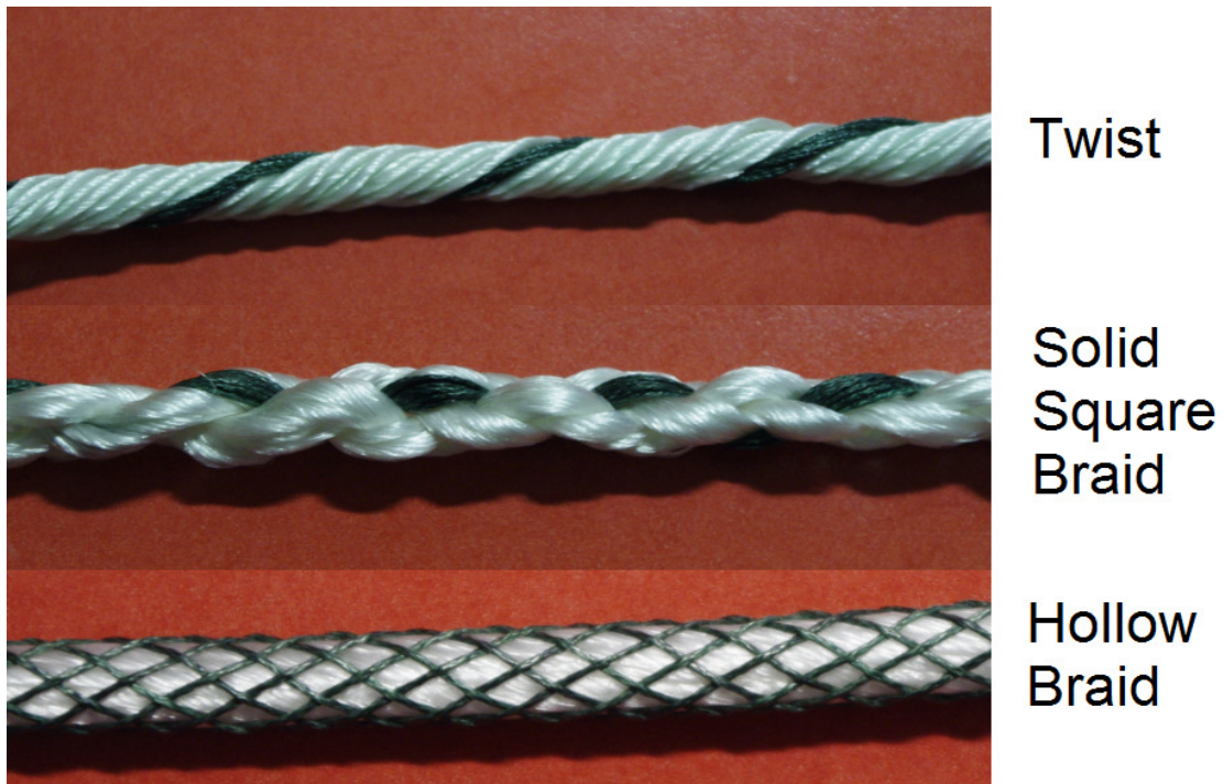
Figure 3.7 Twisted, 4-strand square square braided, and hollow braided samples.
