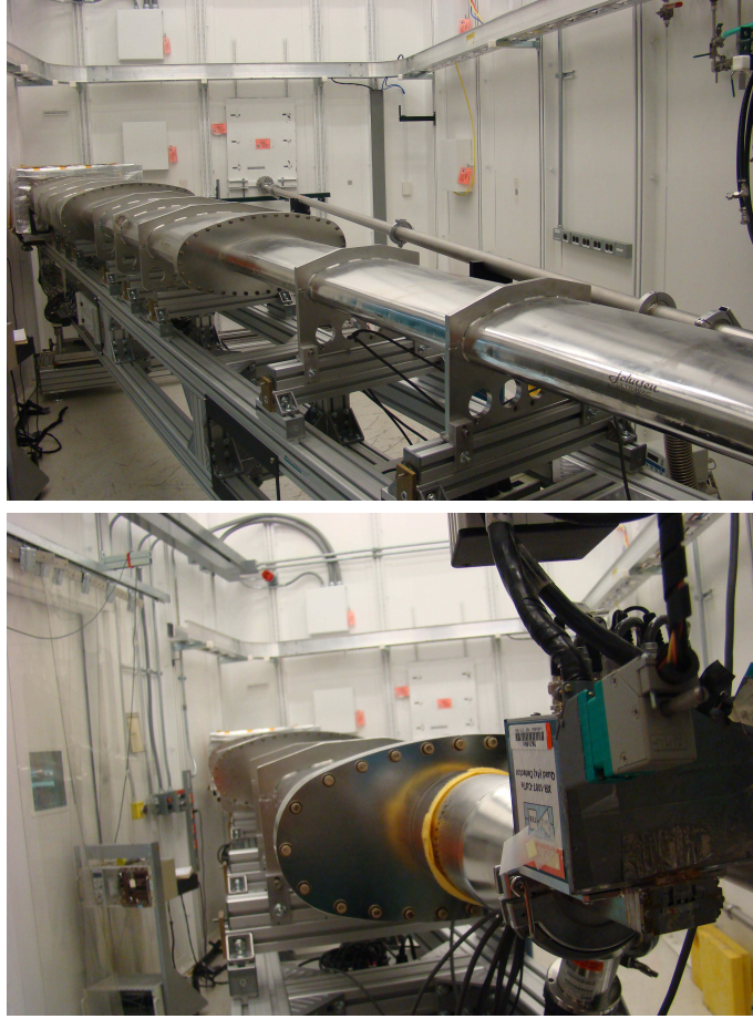
Figure 3.1 Images of sector 3-ID-C of the Advanced Photon Source at Argonne National Laboratory. The top image shows the arm which is moved to adjust 2\theta . At the end are four analyzers, allowing for multiple positions in reciprocal space to be measured at once. The lower figure is taken next to the four-circle goniometer (not shown) and shows the detector which measures the back-scattered beam.
