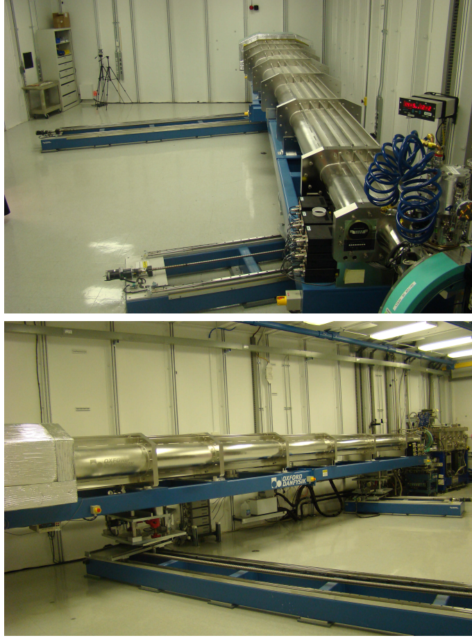
Figure 3.2 Images of sector 30-ID-C of the Advanced Photon Source at Argonne National Laboratory. The top image shows the arm which is moved to adjust 2\theta . At the end are nine analyzers, allowing for multiple positions in reciprocal space to be measured at once. The lower figure is taken from the other side of the room and shows the KB Mirror system and four-circle goniometer.
