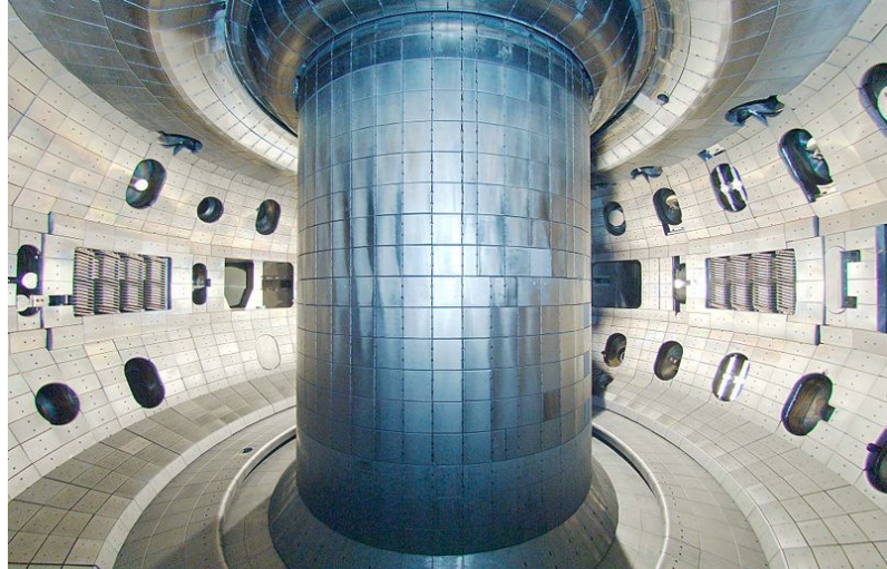
(a) DIII-D interior with diagnostic ports [52]
