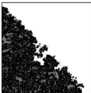
Figure 7. KMC simulation image of interface propagation of the vacuum state (upper right) into the active state (lower left) for h=0 and p=0.100 (above p_e = 0.0944 and close to p_{s+} \approx 0.101 ). Image size: 256 \times 256 sites. The image was taken \sim 800 Monte Carlo steps after the initiation of propagation from a straight interface separating completely filled and empty regions. The image distinguishes empty sites within and connected to the vacuum state (white) from disconnected empty sites and clusters interior to the active state (grey). Occupied sites are black. Note that spontaneous nucleation of the vacuum state occurs within the active state, so that the interior (grey) vacuum clusters grow in time.
