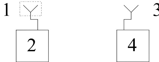
Figure 21. The schematic shield test measurement system. 1. Shield Test Device, 2. Signal Generation Equipment, 3. Receiving Antenna, 4. Signal Detection Equipment
