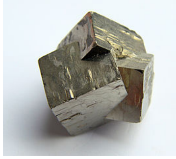
Figure 1.1 A pyrite crystal with simple penetration twinning of three cubic domains.
