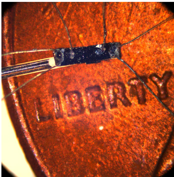
Figure 3.1 A typical sample mounted on the end of a hypodermic needle. Contact leads have been soldered to the sample in a four probe resistivity configuration. A penny in the background gives the reader an impression of the size of a sample.
