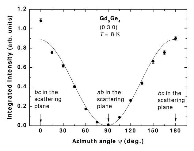
Figure 4.4 The integrated intensity of the  $(0\ 3\ 0)$  magnetic peak normalized by the  $(0\ 4\ 0)$  charge peak at T = 8 K. The solid curve represents the variation expected for magnetic moments along the **c**-axis.
