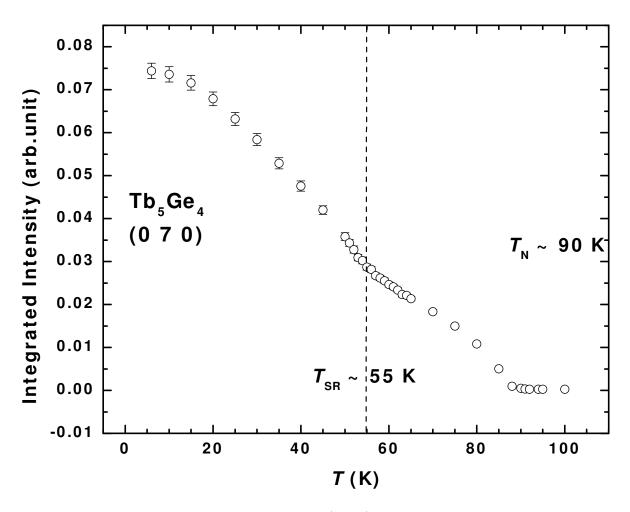
Figure 4.7 Integrated intensity of the  $(0 \ 7 \ 0)$  magnetic reflection measured upon heating the Tb<sub>5</sub>Ge<sub>4</sub> sample.
