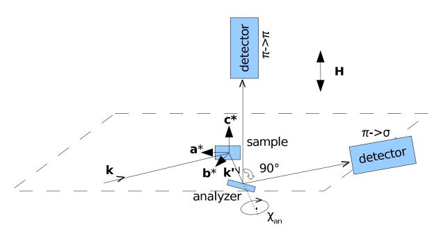
Figure 5.3 The experimental arrangement consisting of the sample, analyzer and detector. **k** and **k'** are the incident and scattered x-ray wave vectors respectively. The magnetic field **H** was applied along the vertical direction. The switch between  $\pi$ - $\sigma$  geometry (the detector arm in the horizontal plane) and  $\pi$ - $\pi$  geometry (the detector arm along the vertical direction) was accomplished by a motor-driven analyzer angle,  $\chi_{an}$ .
