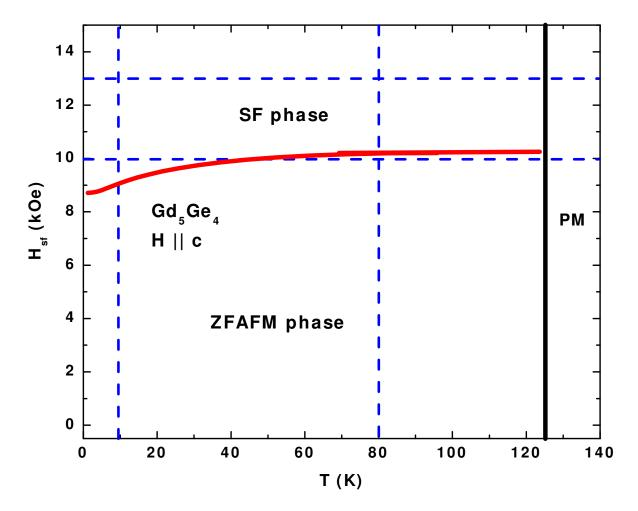
Figure 5.2 Temperature dependence of the spin-flop field,  $H_{\rm sf}$ , derived from the field dependence of the magnetization measured at different temperatures. (From Ref. [OPG<sup>+</sup>06]) PM, SF, and ZFAFM represent the paramagnetic phase, the spin-flop phase, and the zero-field antiferromagnetic phase, respectively. The dashed lines represent the two field-dependence measurements and two temperature dependence measurements using XRMS in the present experiment.
