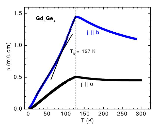
Figure 4.8 The temperature dependence of the electrical resistivity of the  $Gd_5Ge_4$  single crystal measured on heating up the sample with a current applied parallel to the **a** axis and **b** axis respectively. The solid lines are drawn to guide the eyes.
