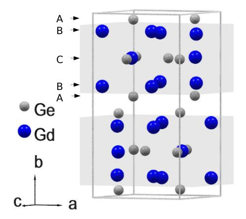
Figure 2.3 The crystal structure of  $Gd_5Ge_4$ . Shaded regions indicate the "slabs" stacked along the **b** direction. The slabs are infinite in the ac plane but they are limited to ~ 7 Å along the **b**-axis. It is interesting to note that each slab consists of five monolayers (ABCBA) stacked along the **b**-axis, originally used by Smith et al [SJT67] to describe the crystallography of the  $Sm_5Ge_4$ -type structure.
