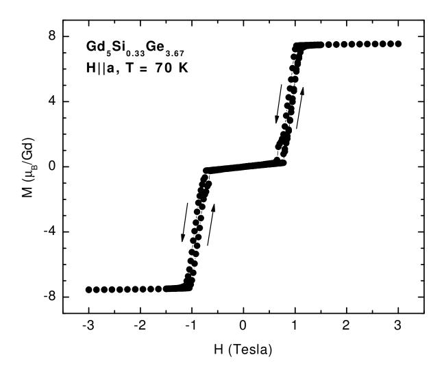
Figure 4.11 The magnetic field dependencies of the magnetization of the zero-field cooled single crystal of  $Gd_5Si_{0.33}Ge_{3.67}$  measured at T = 70 K when the magnetic field vector is parallel to the a-axis. The dashed lines show the extrapolated magnetic behavior without the magnetic field-induced AFM-FM transition during the second field-increasing measurement.
