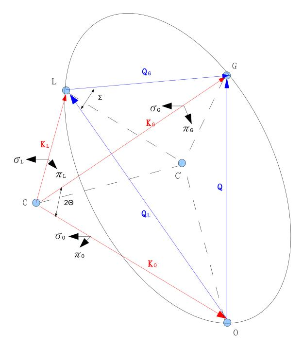
Figure 3.5 Choice of unit polarization vectors  $\sigma$  and  $\pi$  for symmetrical configuration. C denotes the center of the Ewald sphere; C' denotes the center of the optional circle;  $\mathbf{Q}$ ,  $\mathbf{Q}_L$ , and  $\mathbf{Q}_G$  represent scattering vectors. The wave-vectors  $\mathbf{K}_O$ ,  $\mathbf{K}_G$ , and  $\mathbf{K}_L$  lie in a section of Ewald sphere.
