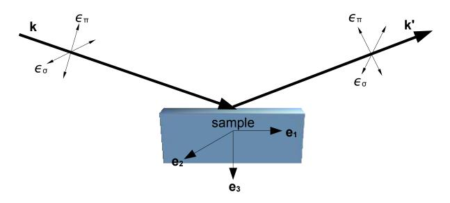
Figure 3.2 The coordinate system used for the polarization dependence of the resonant scattering amplitudes described in the text. **k** and **k'** are the incident and scattered wave vectors.  $\epsilon_{\sigma}$  and  $\epsilon_{\pi}$  are the components of the polarization perpendicular and parallel to the scattering plane. The  $e_2$  axis is perpendicular to the plane of scattering. The  $e_3$  axis is parallel to the scattering vector.
