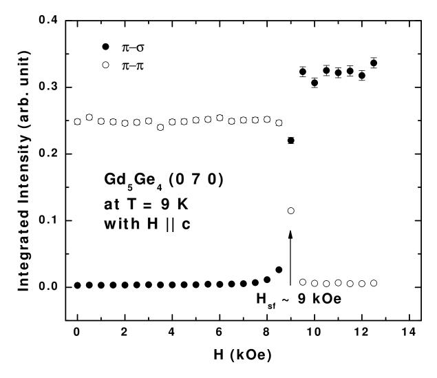
Figure 5.5 The (0 7 0) magnetic reflection measured with increasing magnetic field (along the **c** direction) in both  $\pi$ - $\pi$  and  $\pi$ - $\sigma$  geometries at T = 9 K. Integrated intensity normalized by the (0 8 0) charge reflection.
