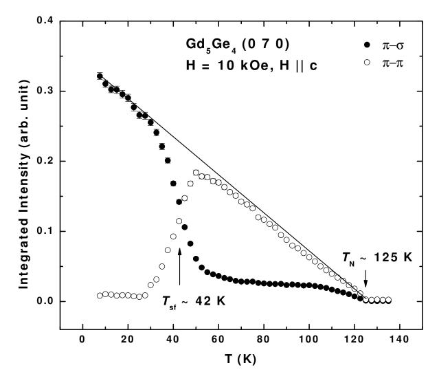
Figure 5.9 Integrated intensity of the  $(0\ 7\ 0)$  magnetic reflection measured when the sample was warmed up in a vertical magnetic field, H = 13 kOe. The data in both scattering channels are normalized by the integrated intensity of the  $(0\ 8\ 0)$  reflection measured in  $\pi$ - $\sigma$ . For comparison, the data in  $\pi$ - $\pi$  are divided by the geometric factor,  $(\sin 2\theta / \cos \theta)^2$ . The straight line is drawn to guide the eyes.
