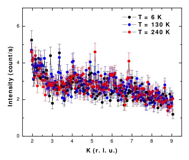
Figure 6.4 The longitudinal K scans, (0 K - 0.2), of  $\text{Gd}_5\text{Ge}_4$  at three different temperatures 6 K (black), 130 K (blue) and 240 K (red) using the analyzer Ge(3 3 3). The counting time for each data point is 20 seconds.
