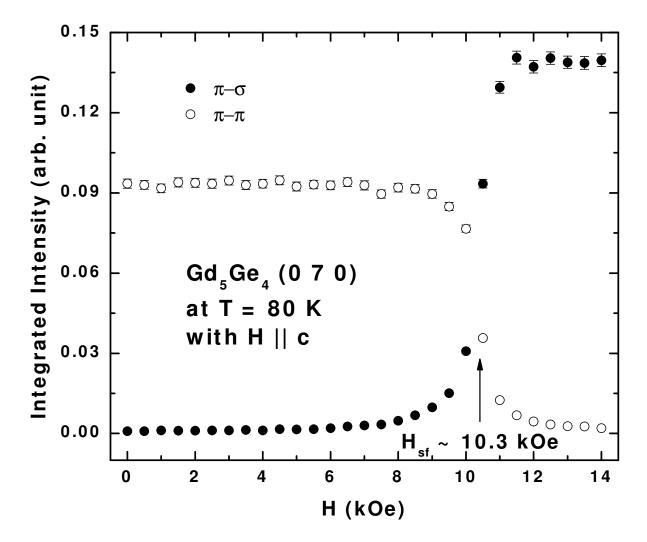
Figure 5.6 The (0 7 0) magnetic reflection measured with increasing magnetic field (perpendicular to the scattering plane) in both  $\pi$ - $\pi$ and  $\pi$ - $\sigma$  geometries at T = 80 K. Integrated intensity normalized by the (0 8 0) charge reflection.
