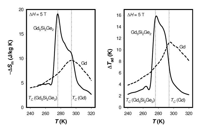
Figure 2.2 MCE curves comparing  $Gd_5Si_2Ge_2$  and Gd. (Left)  $\Delta S_m(T, \Delta H = 5 \text{ Tesla})$  curves; and (right)  $\Delta T_{ad}(T, \Delta H = 5 \text{ Tesla})$  curves. The Curie temperatures of 276 and 294 K, respectively, for  $Gd_5Si_2Ge_2$  and Gd are noted on the MCE curves. The figure is taken from Ref. [Mil06]. Data for these curves were taken from Ref. [PG97b]
