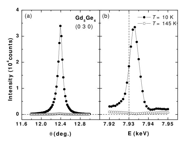
Figure 4.2 (a)  $\theta$  scan through the (0 3 0) magnetic peak at 10 K (filled circles) and 145 K (open circles) and (b) energy scans at 10 K (filled circles) and 145 K (open circles) through the magnetic peak. The data were measured at an azimuth angle of  $\psi = 30^{\circ}$  using aluminum attenuator with 0.41 transmission. The dashed line represents the position of the Gd  $L_{\rm II}$  absorption edge.
