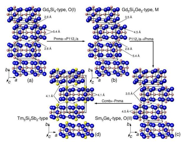
Figure 2.4 Four different types of layered structures found among  $R_5T_4$  compounds: (a) the  $Gd_5Si_4$ -type; (b) the  $Gd_5Si_2Ge_2$ -type; (c) the  $Sm_5Ge_4$ -type; (d) the  $Tm_5Si_2Sb_2$ -type. See the text for a description of differences and relationships among these four structure types. (From Ref. [PG])
