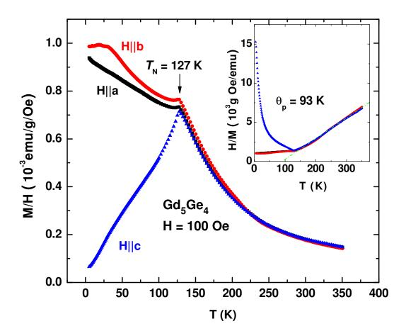
Figure 4.1 Magnetic susceptibility M/H of the  $\mathrm{Gd}_5\mathrm{Ge}_4$  single crystal. The temperature dependence of the susceptibility was measured on heating of the zero-field cooled sample in a field of 100 Oe applied parallel to the three crystallographic axes.
