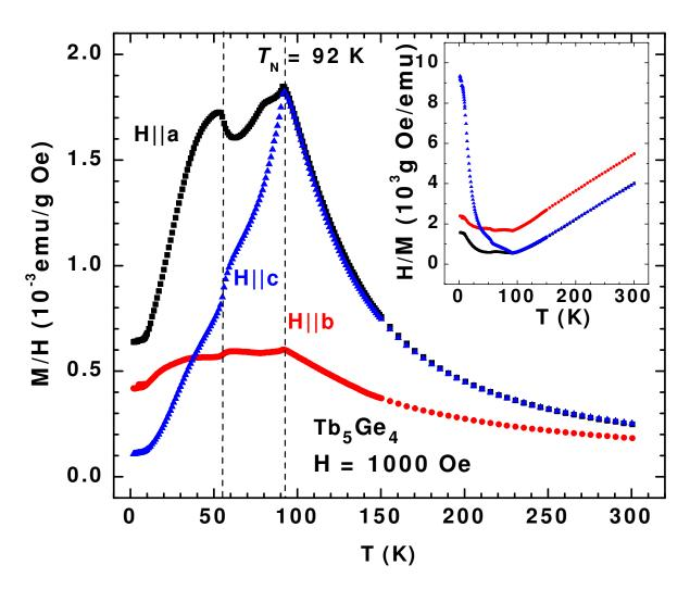
Figure 4.5 Magnetic susceptibility M/H of the Tb<sub>5</sub>Ge<sub>4</sub> single crystal. The temperature dependence of the susceptibility was measured on heating of the zero-field cooled sample in a field of 1000 Oe applied parallel to the three crystallographic axes.
