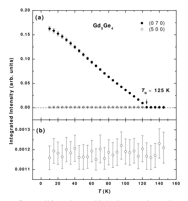
Figure 4.3 (a) Integrated intensity of the (0 7 0) magnetic peak measured upon heating the sample, at an azimuth angle of  $\psi = 30^{\circ}$ , using an aluminum attenuator with 0.41 transmission. (b) Integrated intensity of the (5 0 0) resonant peak measured during heating at an azimuth angle of  $\psi = 60^{\circ}$  without attenuator.
