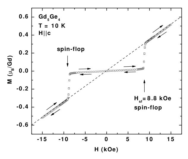
Figure 5.1 Field dependence of the magnetization of a zero-field cooled  $Gd_5Ge_4$  single crystal measured at T = 10 K with the magnetic field parallel to the **c** axis.
