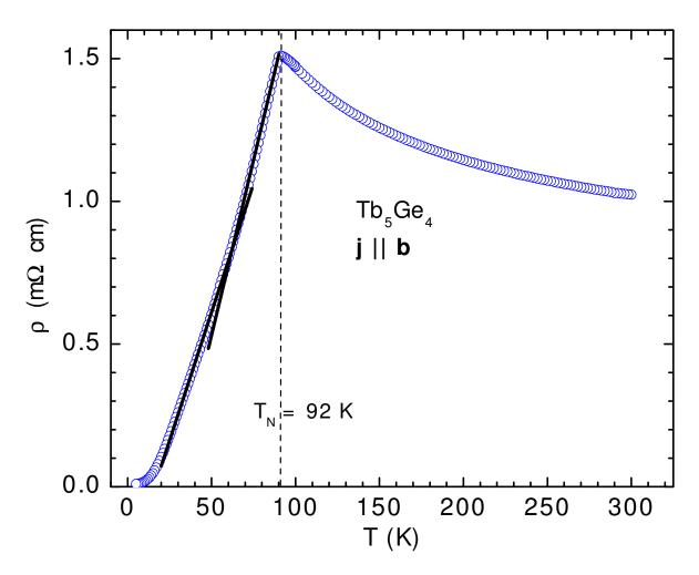
Figure 4.6 The temperature dependence of the electrical resistivity of the  $Tb_5Ge_4$  single crystal measured on heating up the sample with a current applied parallel to the **b** axis. The solid lines are drawn to guide the eyes.
