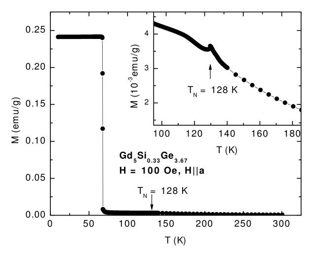
Figure 4.10 The field cooling of the single crystal of  $Gd_5Si_{0.33}Ge_{3.67}$  measured with the magnetic field vector parallel to the a-axis, H = 100 Oe. Inset shows the magnetisation around the Néel temperature (labeled with an arrow).
