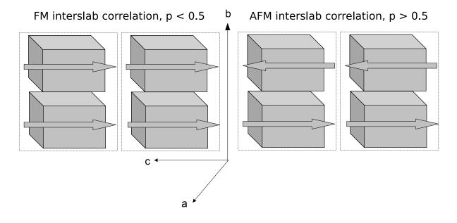
Figure 6.2 Ferromagnetic (left side, high probability when 0 ) andantiferromagnetic (right side, high probability when <math>0.5 )correlations between neighboring slabs in the Hendricks-Tellerpartial order.
