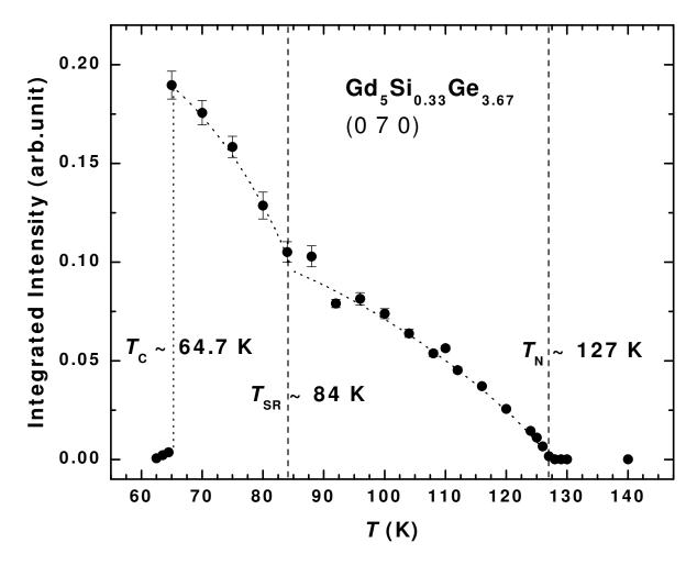
Figure 4.12 Integrated intensity of the  $(0\ 7\ 0)$  magnetic reflection measured upon heating the Gd<sub>5</sub>Ge<sub>4</sub> sample. The data is normalized by the  $(0\ 8\ 0)$  charge reflection. The dotted lines are drawn to guide the eyes.
