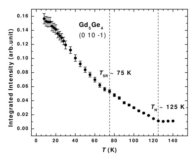
Figure 4.9 Integrated intensity of the  $(0 \ 10 \ -1)$  magnetic reflection measured upon heating the  $Gd_5Ge_4$  sample.
