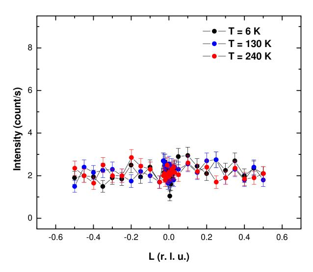
Figure 6.6 The transverse L scans, (0 8.65 L), of  $Gd_5Ge_4$  at three different temperatures 6 K (black), 130 K (blue) and 240 K (red) using analyzer  $Ge(3 \ 3 \ 3)$
