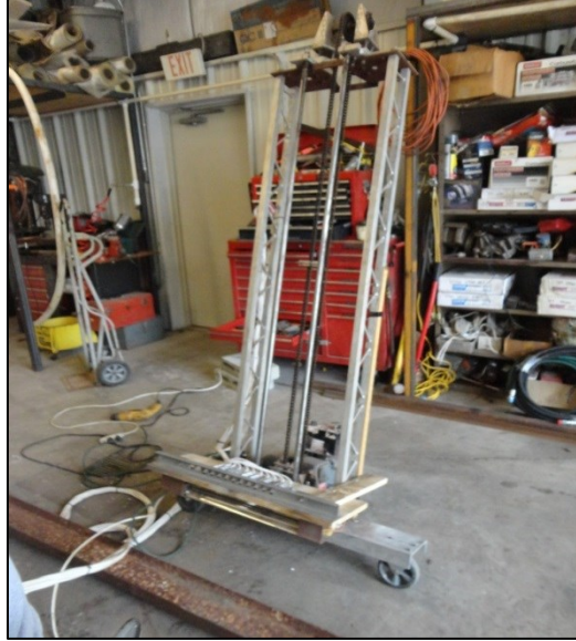
Figure 3b: Photograph of Thermal Scanner
