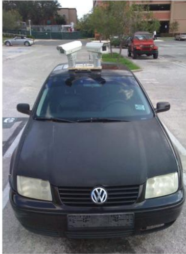
(a) Roadway Video Log Surveillance system (RVLS)
