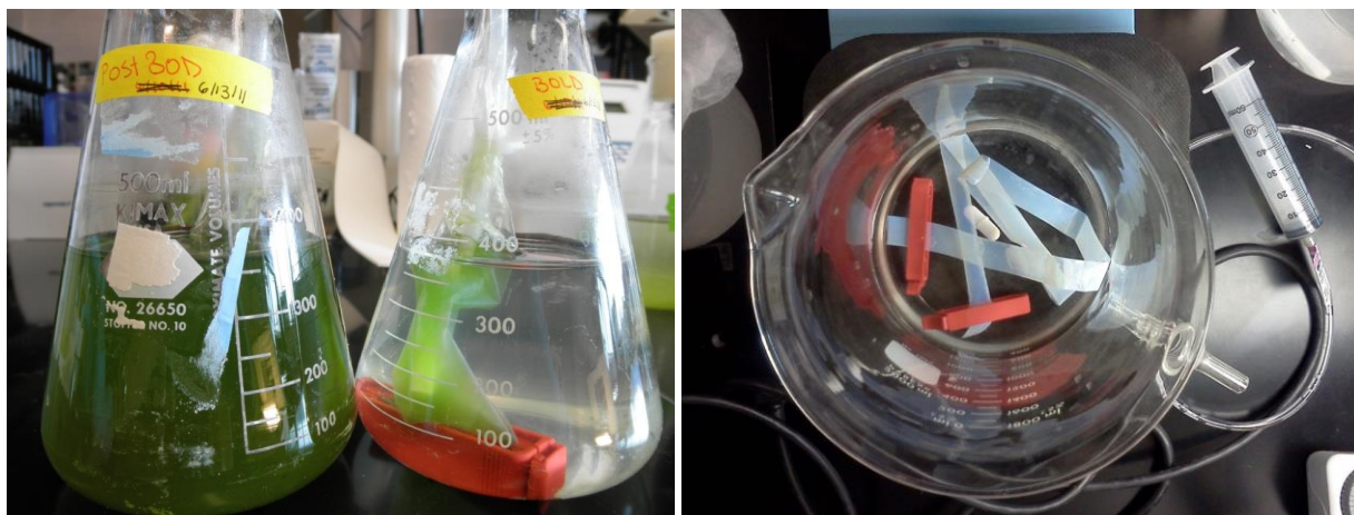
Figure A1. Experimental set ups for preliminary ICARUS tests using dialysis bags of regenerated cellulose and cellulose acetate. Photographs courtesy of Breeyn Greer.
