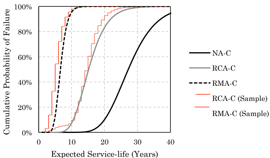
Figure 9 - Graph showing the sample data plotted next to the lognormal distribution produced using the lognormal mean and standard deviation of the sample data. The Anderson Darling test used these plots to validate the lognormal distribution of the data.
