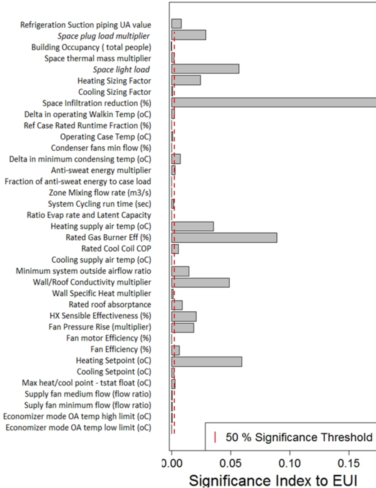
Figure 32: Results of OAT parameter pre-screening for effect on total energy use (EUI)
