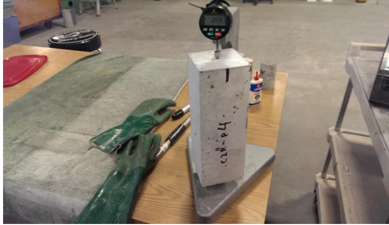
Figure 98 – Taking length comparometer readings of a concrete prism.
