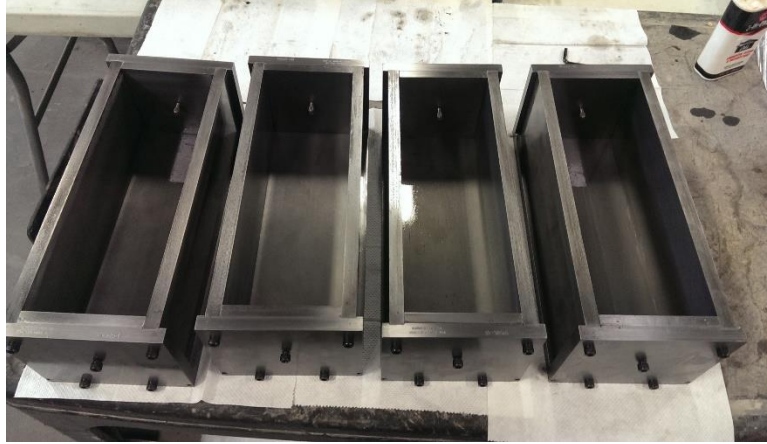
Figure 94 - 4-inch square prism molds ready for casting
