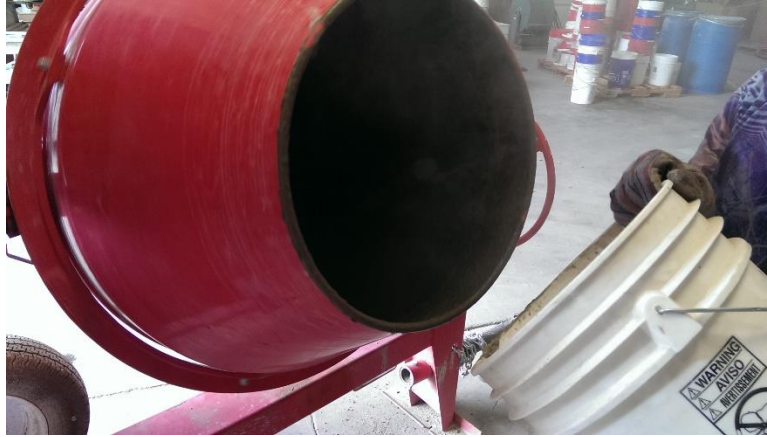
Figure 76 - Charging the mixer
