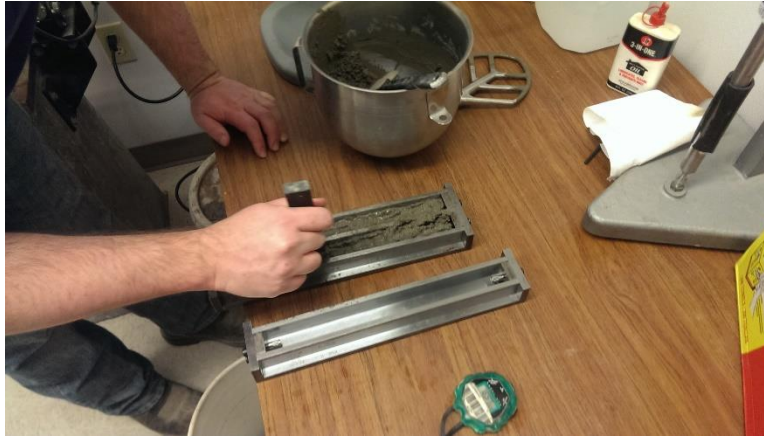
Figure 48 - Tamping mortar into molds
