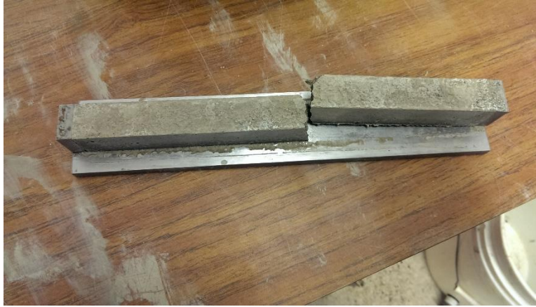
Figure 50 – This mortar bar broke during extraction
