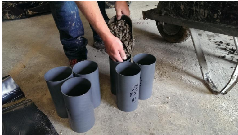
Figure 87 - Filling compression test cylinder molds
