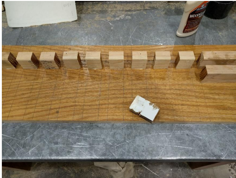
Figure 21 - Joining wooden blocks to jig base with wood glue and steel brad nails.
