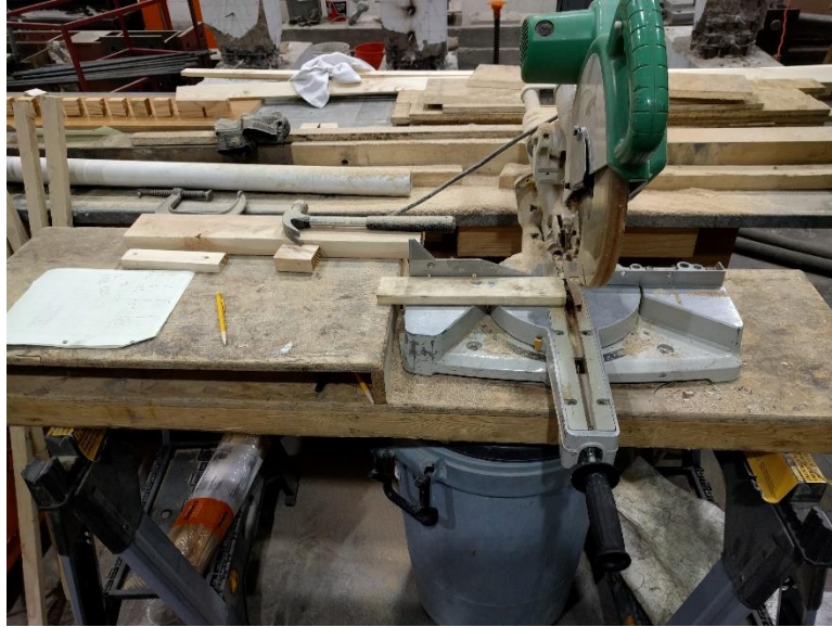
Figure 19 - Cutting wooden blocks for the welding jig.
