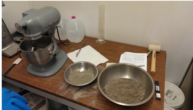
Figure 46 – Mixer with measured cement, water, and aggregate
