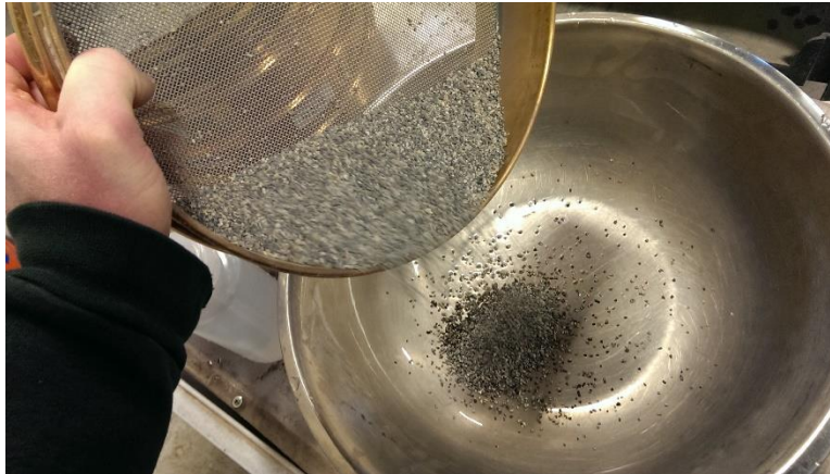
Figure 40 - The contents of each sieve were separated into steel bowls.
