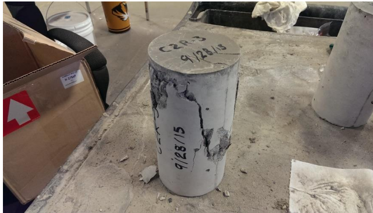
Figure 93 - Fractured cylinder after testing
