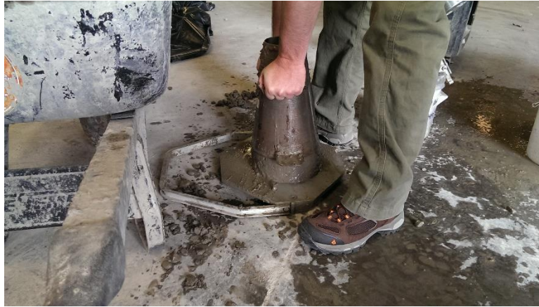
Figure 81 - The slump mold is lifted in one smooth motion.
