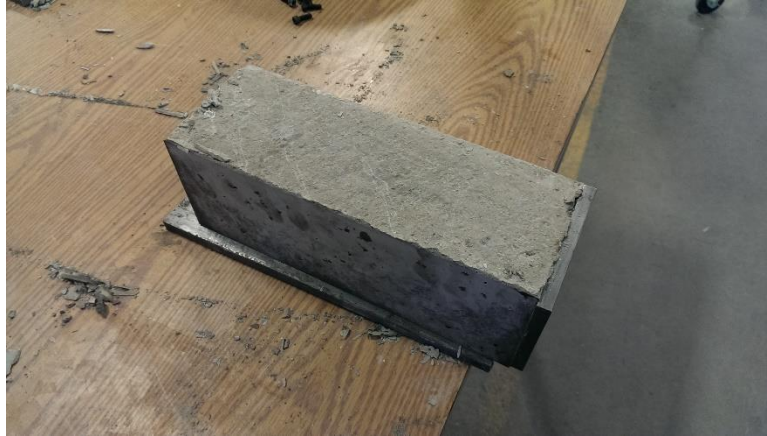
Figure 96 - Demolding a concrete prism.
