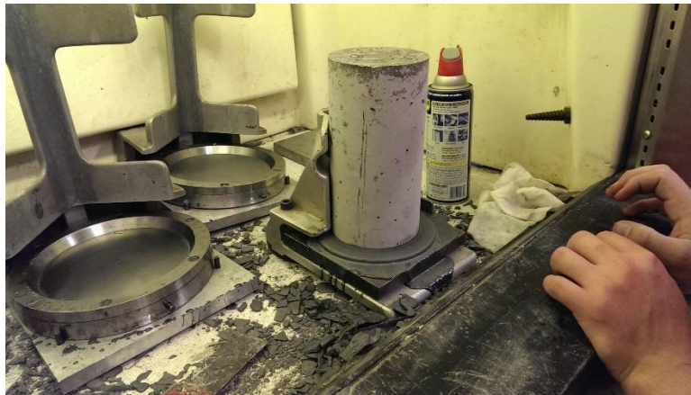
Figure 91 - Installing sulfur mortar end caps
