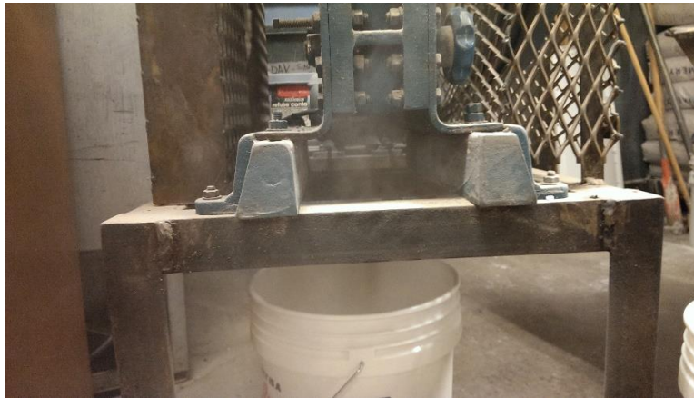
Figure 38 - Aggregate crusher in use at University of Colorado materials laboratory
