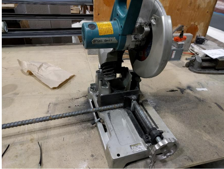
Figure 22 - Cutting reinforcing bar
