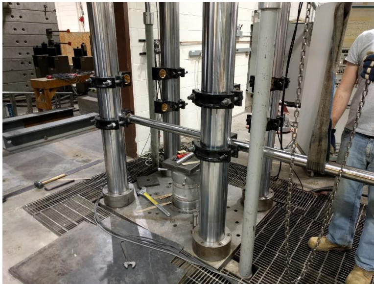
Figure 11 - Bushing clamps are installed on the vertical columns of the MTS hydraulic press.
