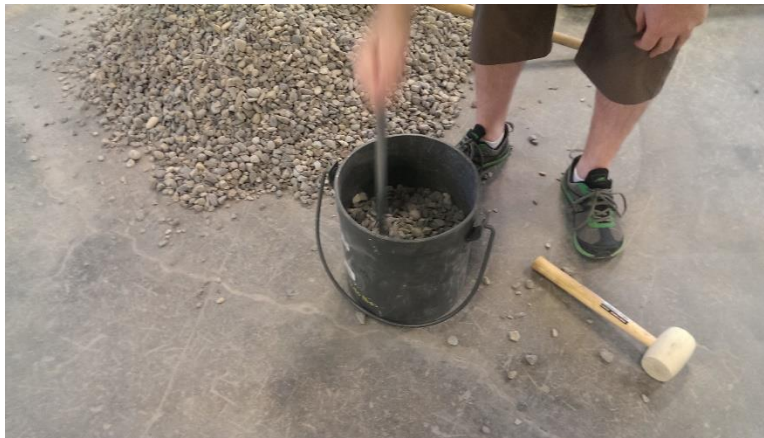
Figure 70 - Each lift is rodded 25 times.
