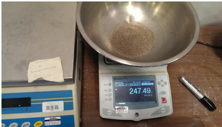
Figure 43 - Balance used to weigh dried aggregate
