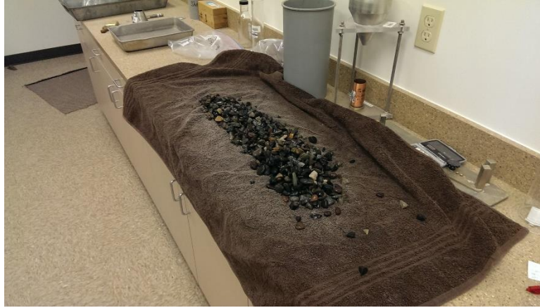
Figure 60 - Soaked coarse aggregate is spread on a towel for drying to saturated surface-dry condition.
