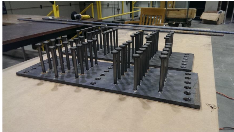
Figure 8 - Sample end plates with shear studs
