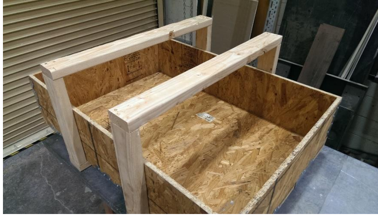
Figure 26 – Example shear specimen formwork
