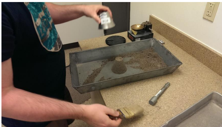
Figure 65 - Saturated surface-dry conditions are reached when sample slumps slightly when cone mold is removed. This sample does not slump and is still too wet.
