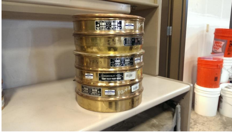
Figure 72 Sieve stack ready for coarse aggregate analysis
