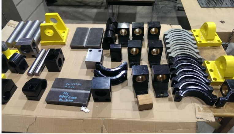
Figure 10 - Components of the shear test apparatus were cleaned and painted prior to assembly.
