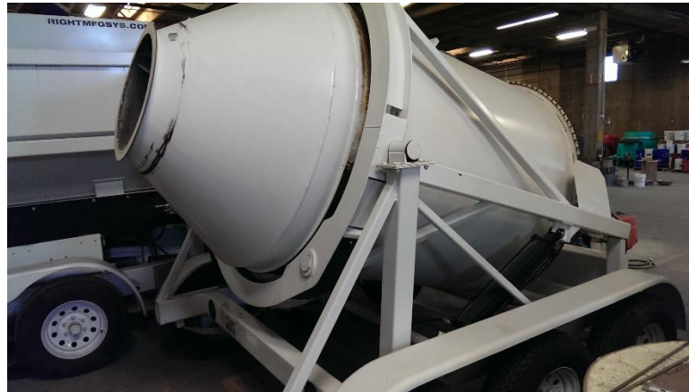
Figure 28 - The three-cubic yard mixer at Fall Line
