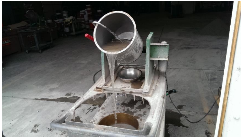
Figure 71- Washing aggregate in preparation for sieve analysis
