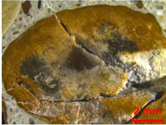
Figure 1 – ASR damage in chert coarse aggregate.
