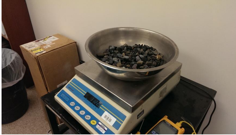
Figure 62 - Coarse aggregate at SSD is weighed
