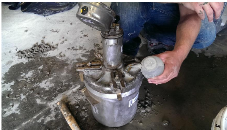
Figure 86 - A small quantity of water and isopropyl alcohol is added just until it begins to run out the weep hole.
