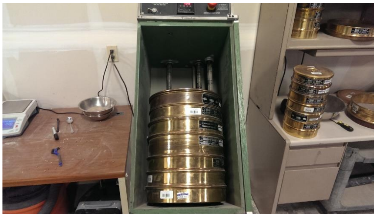
Figure 39 - Mechanical shaker with sieves at Fall Line laboratory
