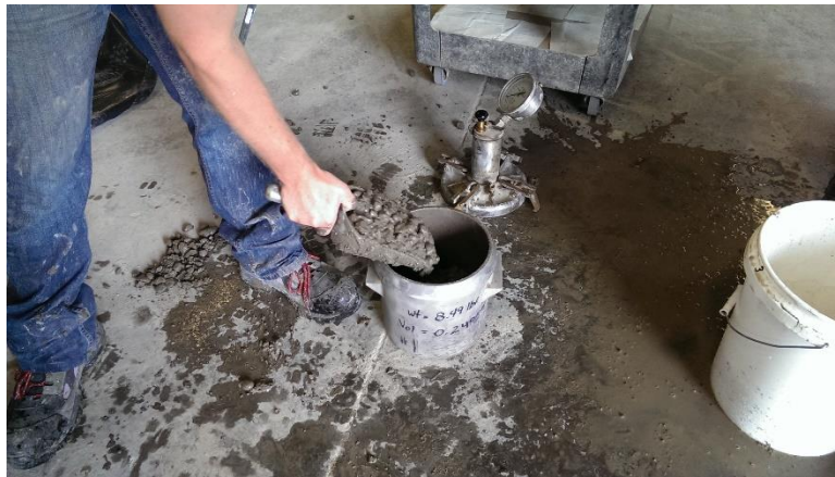
Figure 83 – The air meter bowl is filled in two layers, each rodded 25 times.
