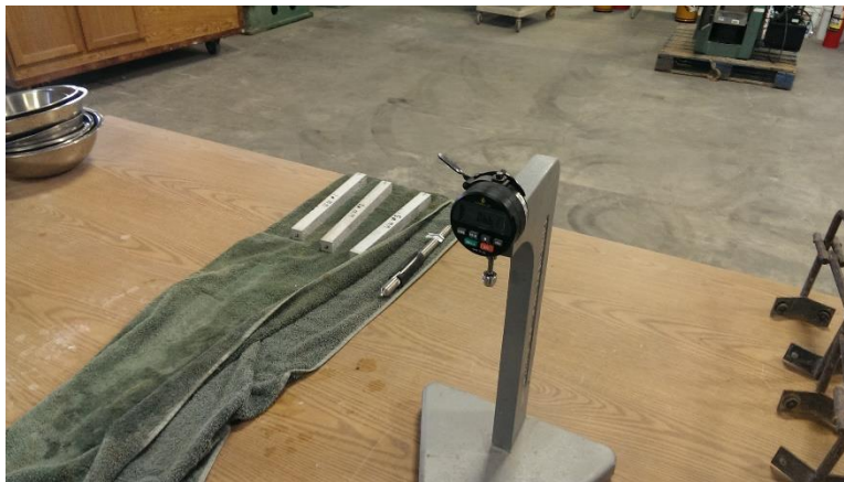
Figure 51 - Initial readings were taken before bars were placed in water bath.
