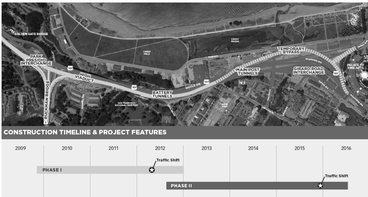
Figure 3: Presidio Parkway Construction Overview (Source: www.presidioparkway.org )
