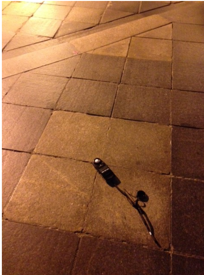
Figure 5.2: Horizontal Illuminance Measurements
