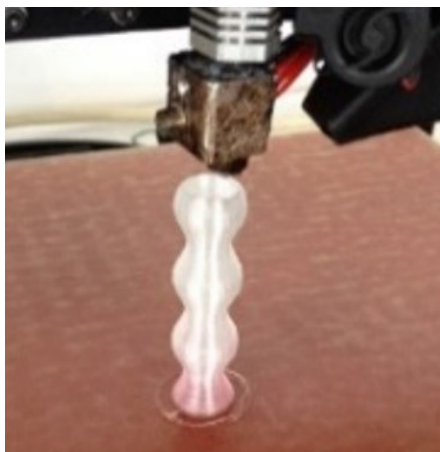
Figure 8.2: Printing of a tortuous channel with t-glase filament in a Lulzbot printer
